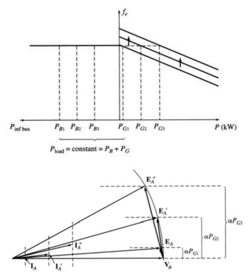
Note an increase in power (with V<sub>t</sub> and E<sub>A</sub> staying constant), results in an increase in the power angle δ.
