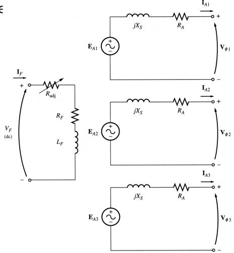
A synchronous generator can be Y- or  $\Delta$ -connected:
