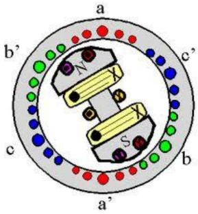
The rotor of a synchronous machine is a large electromagnet. The magnetic poles can be either salient (sticking out of rotor surface) or non-salient construction.
