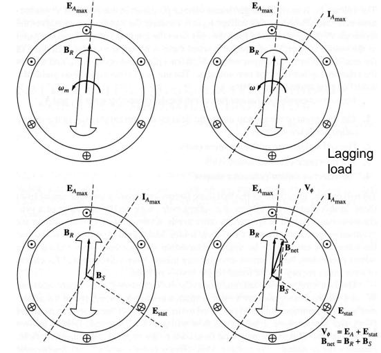
The load current  $I_A$  will create a stator magnetic field  $B_S$ , which will produce the armature reaction voltage  $E_{stat}$ . Therefore, the phase voltage will be
