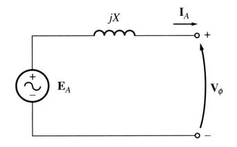
However, in addition to armature reactance effect, the stator coil has a self-inductance  $L_A$  ( $X_A$  is the corresponding reactance) and the stator has resistance  $R_A$ . The phase voltage is thus
